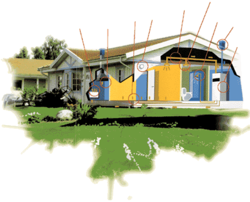
Picture 7. Exhaust heat pump is changing the air volume of the house once in two hours and recovering the heat from outlet air. Recovered energy is used for warming up water for distribution and tap water system.
